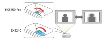
If your image looks like \_\_\_\_ or \_\_\_\_, you may have placed the projector off to one side of the screen at an angle. Place the projector directly in front of the center of the screen, facing the screen squarely. If you can't move the projector, use the horizontal keystone slider on the projector to correct the image shape.
