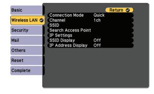
Choose **Connection Mode**, press \(\frac{1}{2}\), select **Quick** for a direct connection to a computer, tablet, or smartphone, then press \(\frac{1}{2}\) again. When you're finished, press **Esc** to return to the Wireless LAN menu.
